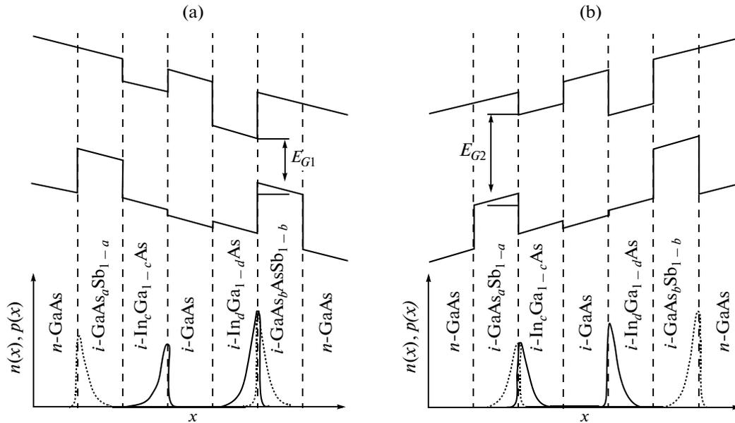
**Fig. 2.** Band diagrams of (a) first and (b) second versions of frequency modulator nanostructure and corresponding distributions of (solid lines) electron concentration and (dashed lines) hole concentration at opposite directions of control field.
