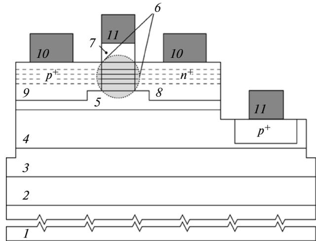
**Fig. 1.** Structure of an injection laser with a functionally integrated frequency modulator: (1) silicon substrate, (2) buffer gradient GaAsP layer [10], (3) semi-insulating GaAs, (4)  $p$ -GaAs, (5)  $n$ -GaAs, (6) frequency-modulator nanoheterostructure, (7)  $n$ -GaAs, (8) injecting  $n^+$  domain, (9) injecting  $p^+$  domain, (10) feed contact, and (11) control contact.
