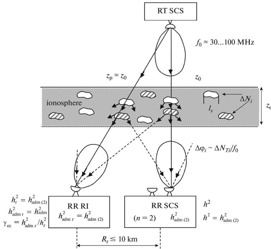
Fig. 1. Transionospheric radio wave propagation at low SCS carrier frequency ( $f_0 = 30\text{--}100$  MHz).
