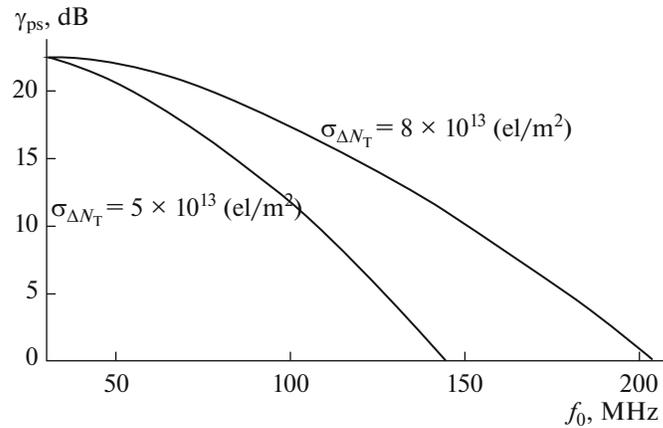
Fig. 4. Dependence of SCS energy concealment factor on selection of carrier frequency using dual signal reception.
