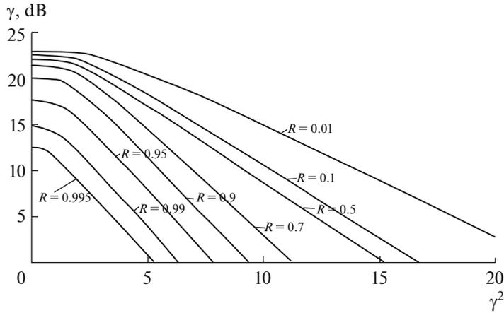
Fig. 2. Dependence of SCS energy concealment factor on both fade depth and fading spatial correlation coefficient of antennas.
